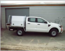
Ranger with full toolbox, front & rear ladder rack
