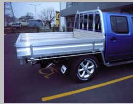
Galvanised deck with alloy sides & alloy floor
